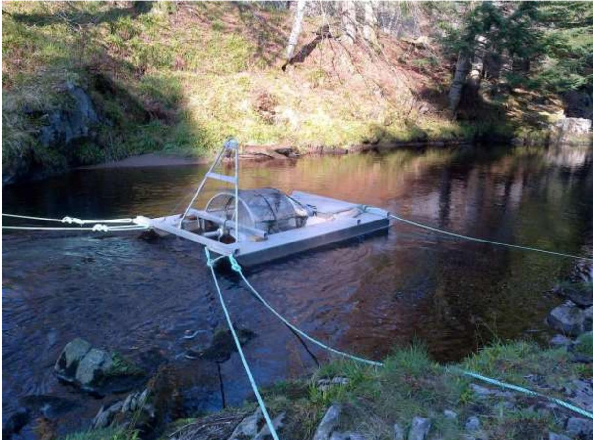
*Rotary screw trap in place on the River Divie during spring 2017.*
